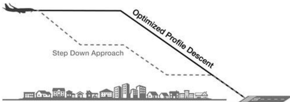
Under traditional staircase descent procedures, aircraft repeatedly level off and power up the engines. This burns more fuel and requires air traffic controllers to issue instructions at each step. With optimized descents, aircraft descend from cruising altitude to the runway in a smooth, continuous path with the engines set at near idle.
