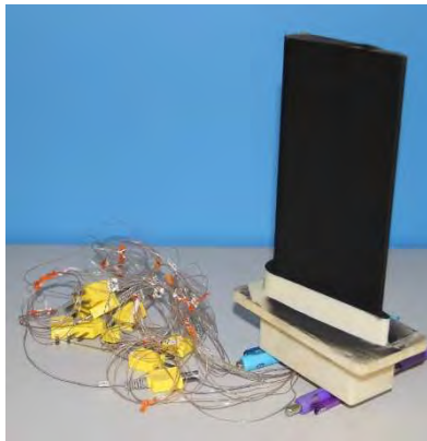
Figure 4-4. Flow Visualization and Calibration Airfoil
