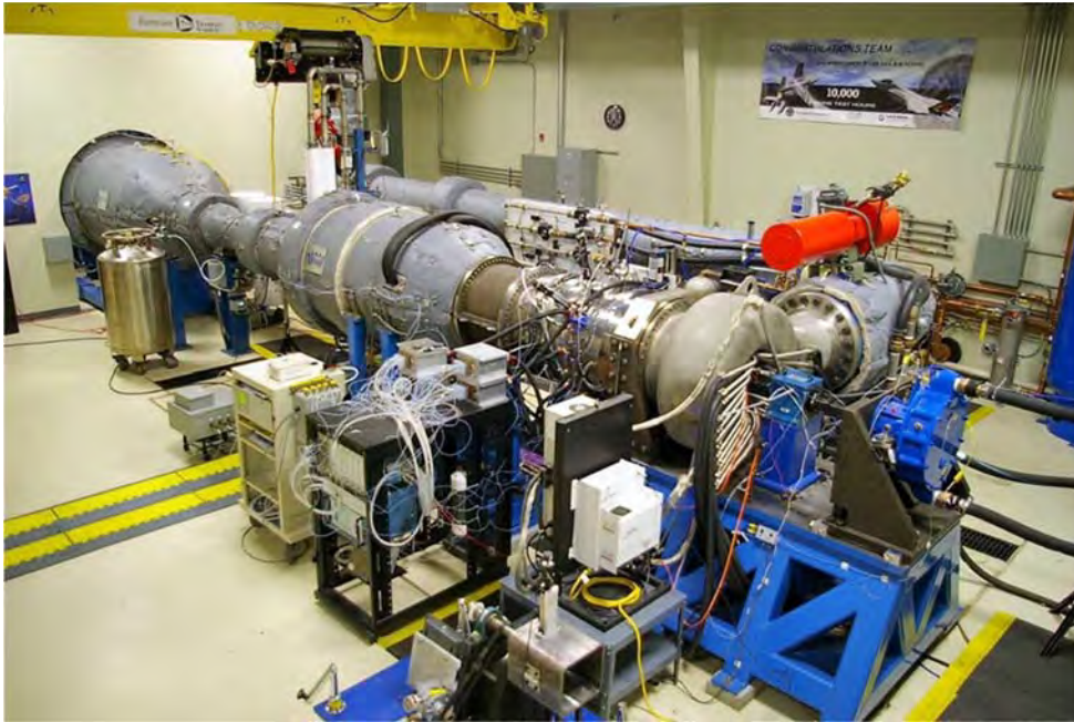
Figure 2-14. An Overview Photograph of the Turbine Room Taken During the Testing Campaigns Showing the Rig and Many of the Test Section Components Including Instrumentation Systems. Image credit: PSU
