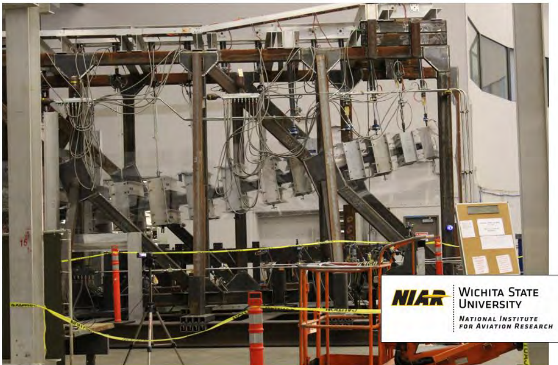
Figure 8 SEW WCTA Test to 177% Design Limit Load
